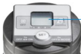
Reusable DRIVE BOOSTER control unit LCD display for setting function and discharge period
