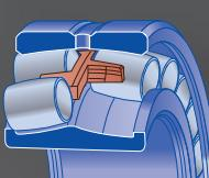
Single-piece cage with reduced bore, external diameter and radial clearance tolerances
