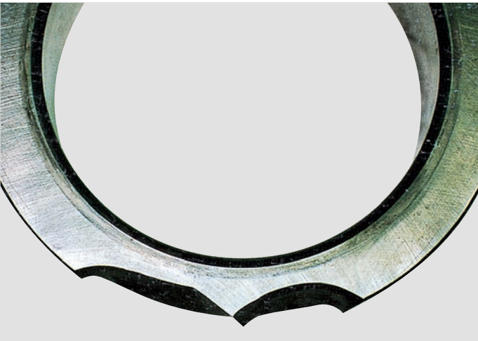
Photo C-3 • Tapered roller bearing inner ring • Extensive chipping of collar • Caused by impact due to poor assembly
