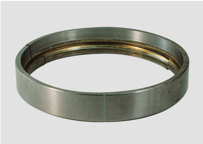
Photo D-4 • Angular bearing outer ring • Fracture in the circumferential direction of the raceway surface • Caused by ball slipping due to poor lubrication
