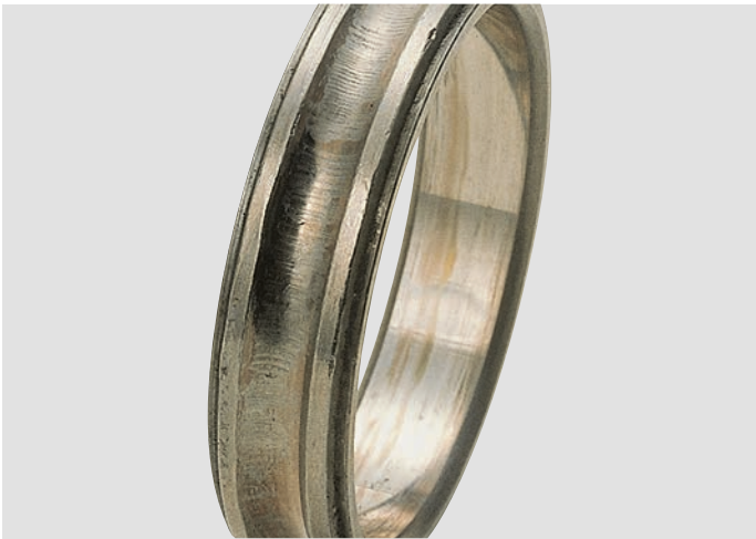
Photo F-2 • Deep groove ball bearing inner ring • False brinelling has occurred around the total circumference of the raceway surface • Caused by vibration
