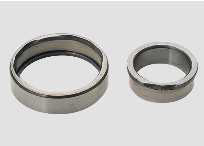
Photo C-1 • Cylindrical roller bearings • Chipping of inner/outer ring guide collar • Caused by excessive impact load
