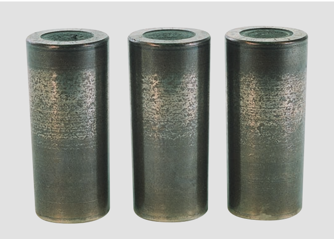
Photo B-3 • Tapered roller bearing rollers • Indentation has occurred on the raceway surface (temper coloration at both ends) • Caused by intrusion of foreign material in the lubricant
