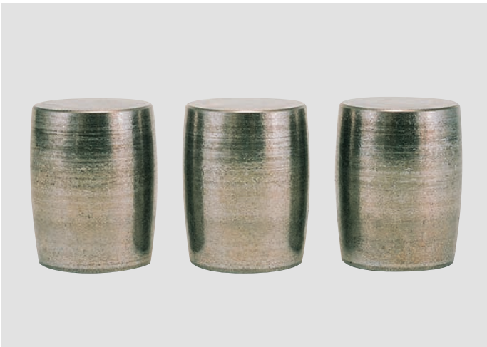
Photo B-2 • Spherical roller bearing rollers • Indentation has occurred on the raceway surface • Caused by the compaction of solid foreign material
