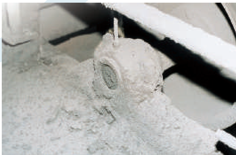
Pulley bearing in extreme contamination conditions (Plummer block)
