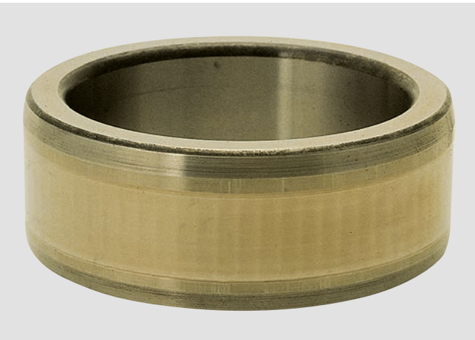
Photo F-1 • Cylinder roller bearing inner ring • False brinelling has occurred around the total circumference of the raceway surface • Caused by vibration
