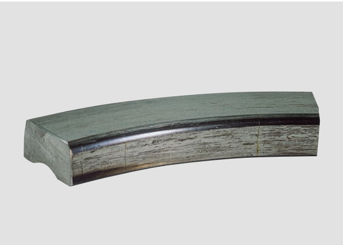
Photo G-3 • Thrust ball bearing shaft washer • Scoring and also friction cracking have occurred caused by bore surface creep
