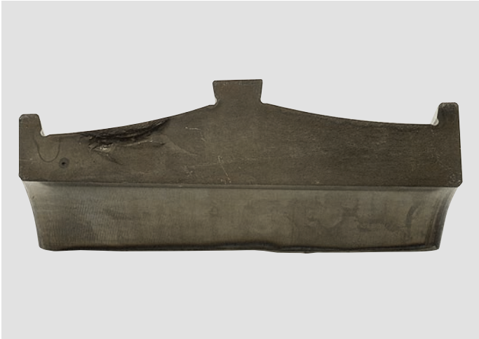
Photo D-2 • Photo D-1 fracture surface • Source in the mid-section of the left-side raceway surface
