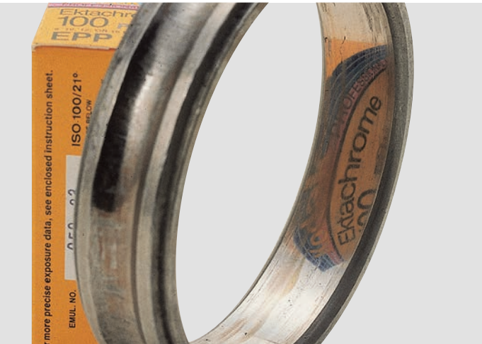
Photo G-1 • Deep groove ball bearing inner ring • Mirroring has occurred on the bore surface due to creep
