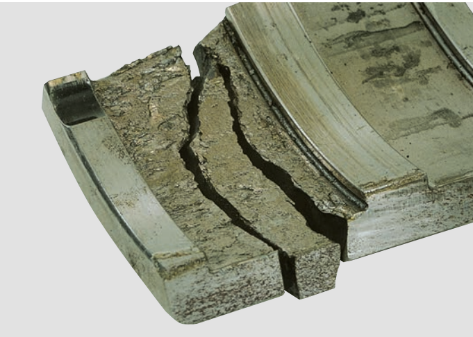
Photo D-3 • Four row cylinder roller bearing outer ring • Fracture in the circumferential direction of the raceway surface • Excessive flaking is the source of fracturee
