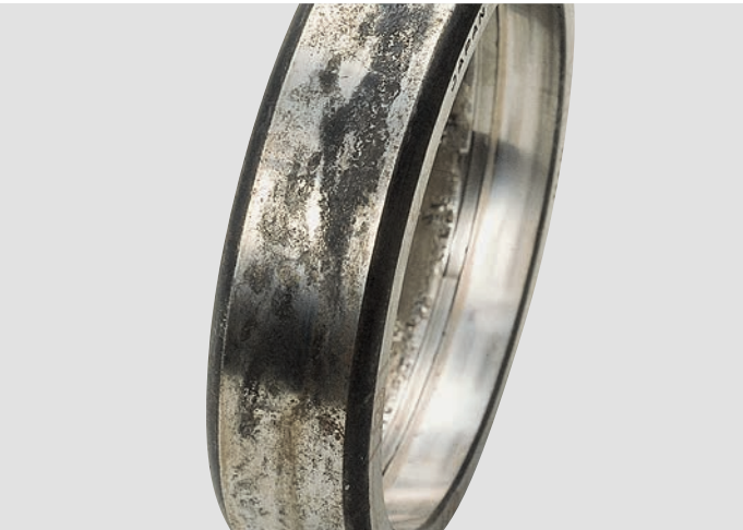
Photo F-3 • Cylinder roller bearing outer ring • Fretting corrosion has occurred along the outer diameter
