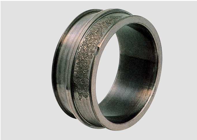
Photo A-4 • Spherical roller bearing inner ring • Flaking has occurred only on one side of the raceway surface • Caused by excessive axial load
