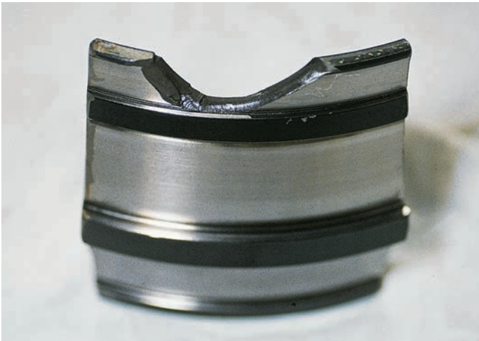
Photo C-4 • Double row tapered roller bearing inner ring • End surface chipping • Caused by impact due to poor bearing handling
