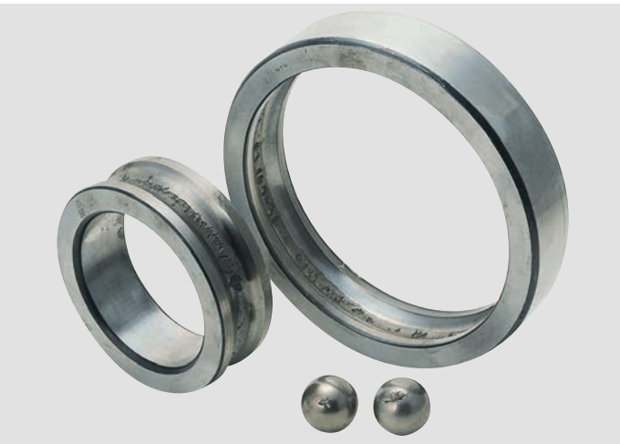
Photo A-1 • Deep groove ball bearings • Flaking has occurred on each of the inner/outer ring and balls • Caused by excessive load
