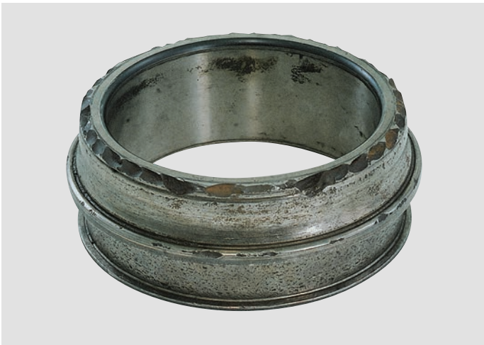
Photo C-2 • Spherical roller bearing inner ring • Chipping of collar section • Caused by excessive impact load
