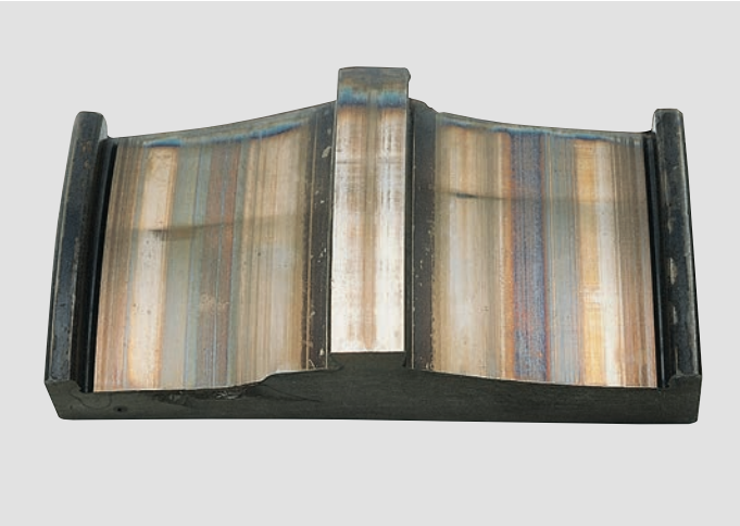
Photo D-1 • Spherical roller bearing inner ring • Fracture of the raceway surface in the axial direction • Caused by excessive interference fit
