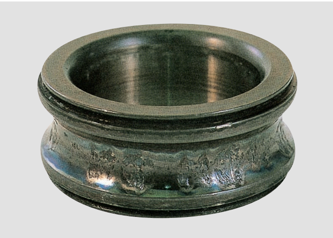
Photo A-3 • Deep groove ball bearing inner ring • Flaking has occurred on one side of the raceway surface • Caused by excessive axial load
