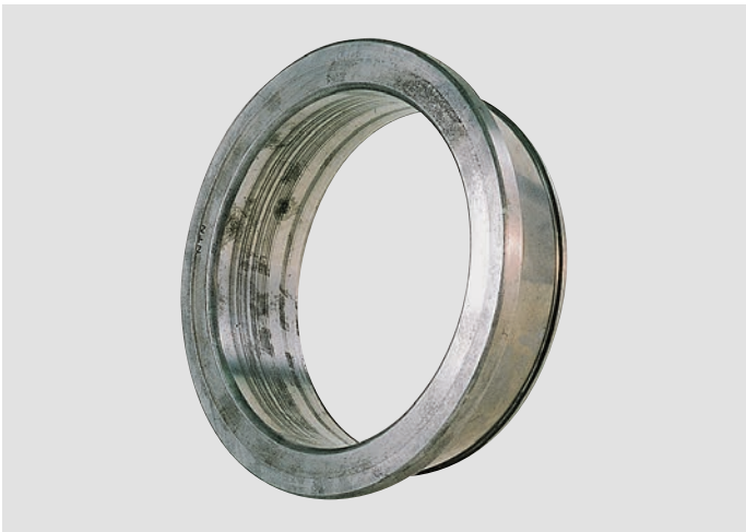
Photo G-2 • Tapered roller bearing inner ring • Scoring caused by creep has occurred in the center section of the bore surface
