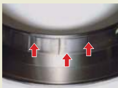
Excessive wear occurred
